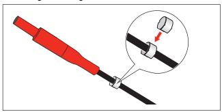
Figure 1. Cable Marker Clips
