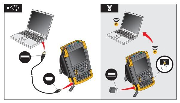
Figure 1. Test Tool to PC Connections
