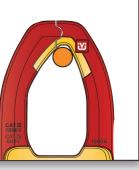
The display shows (a) to indicate that the measurement is from the jaw. When the current measurement is < 0.5 A, the center dot in the icon flashes. For current measurements > 0.5 A, the center dot in the icon is steady.
