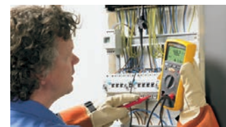
Insulation test at a distribution panel
